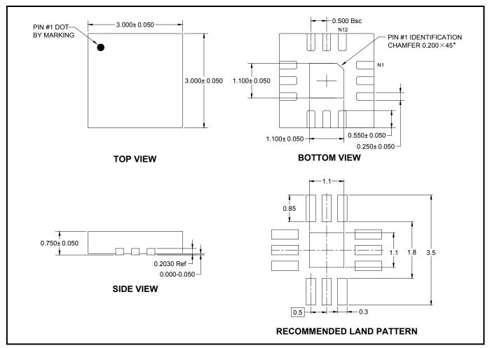
NOTE: All linear dimensions are in millimeters.
